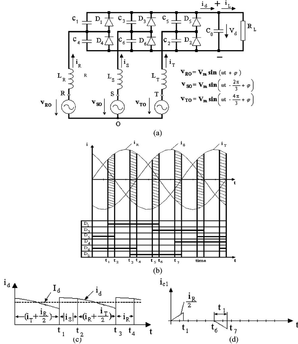
Fig. 2. Three-phase rectifier with near sinusoidal input currents (RNSIC converter). (a) New configuration. (b) AC current waveforms. (c) DC current  $i_d$ . (d) Waveform of the capacitor current  $i_{c1}$ .
