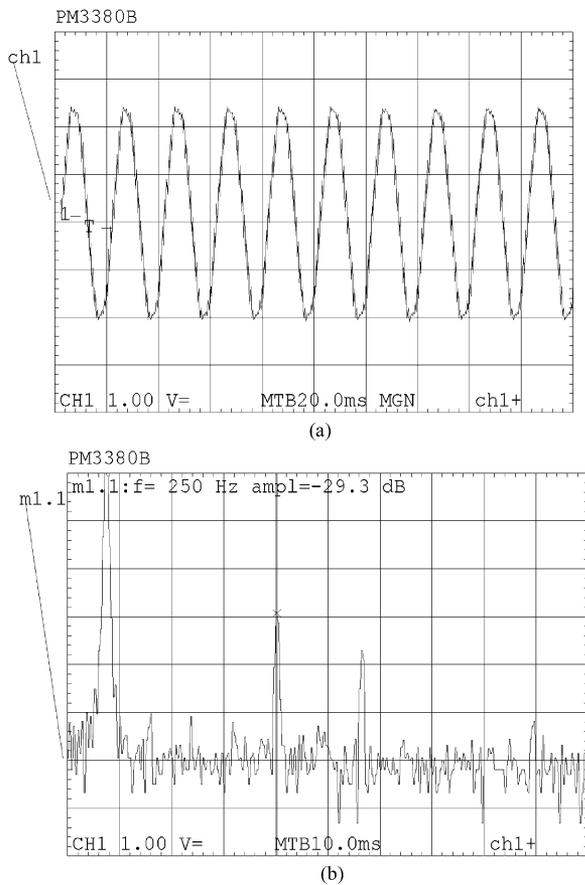
Fig. 10. Experimental results for  $L = 20$  mH,  $C = 40$   $\mu$ F, and  $R_L = 60$   $\Omega$ . (a) Waveform of the phase current. (b) Spectrum of the phase current.
