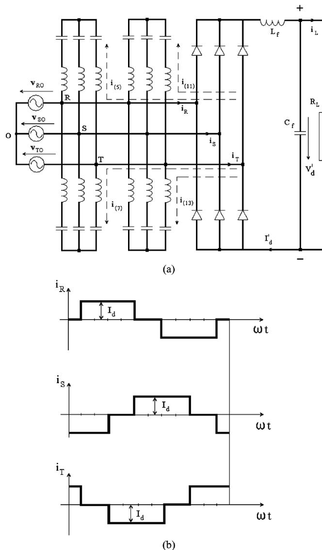
Fig. 1. Three-phase six-pulse full-bridge diode rectifier with passive filters. (a) Classical configuration. (b) Current waveforms.
