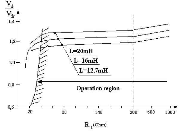
Fig. 6. Variations of the ratio  $V_d/V_{dr}$  as a function of  $R_L$  and  $L$ .
