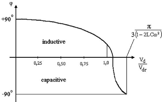
Fig. 4. Variation of the angle  $\varphi$  as a function of the ratio  $V_d/V_{dr}$ .
