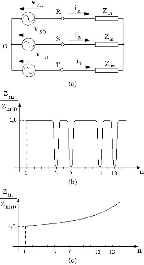
Fig. 3. Simplified equivalent circuit for ac–dc converter (a) Configuration. (b) Variation of the ratio  $Z_{in}/Z_{in(1)}$  in the classical configuration. (c) Variation of the ratio  $Z_{in}/Z_{in(1)}$  in the RNSIC converter.
