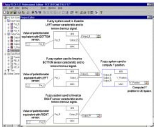
**Fig. 8.** Structure of the Fuzzy Logic system
