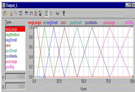
Fig. 5. Output membership functions of the first fuzzy system
