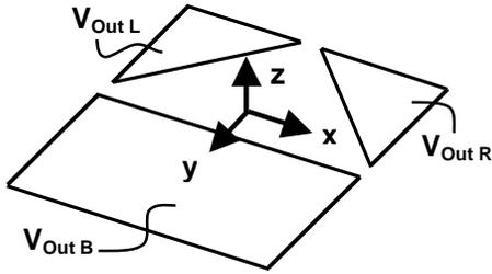
**Fig. 2.** Cartesian co-ordinate system associated with the sensors (in all paper: L – left, R – right, B – bottom);
