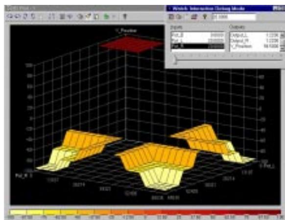
**Fig. 9.** Fuzzy characteristic surface for zero output value of the bottom sensor
