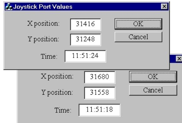
Fig. 6. The value read from the Joystick port at two different moments with a constant value of the both resistors
