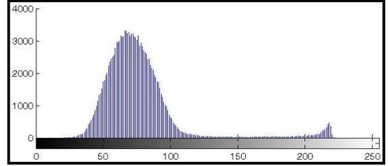
Figure 1 (c) Image processing stages - the histogram of the grayscale image
