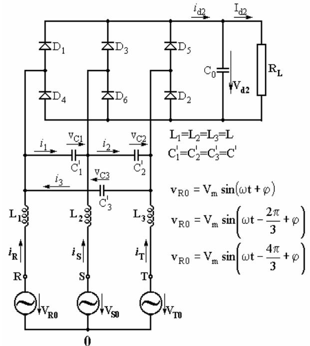
Fig.3. RNSIC converter with capacitors on the AC side
