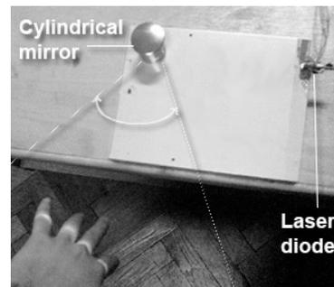
Fig. 1 Laser system with cylindrical mirror
