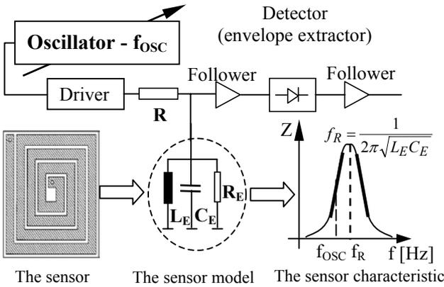
Figure 1: The sensor and the driver circuit
