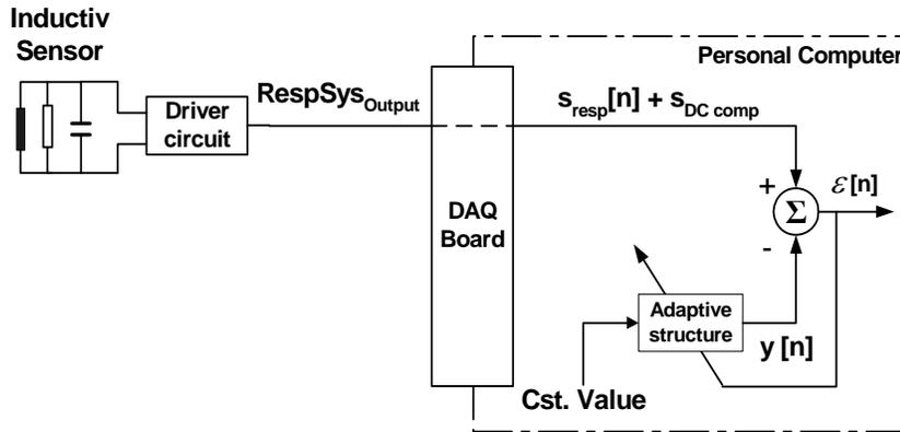
Figure 5 - The implemented structure of the adaptive system
