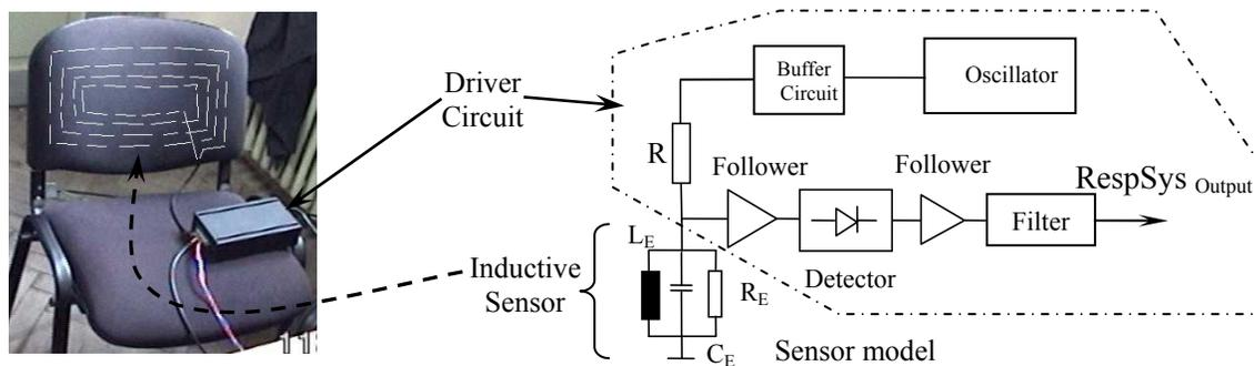
Figure 1 - The respiratory acquisition system and the driver circuit
