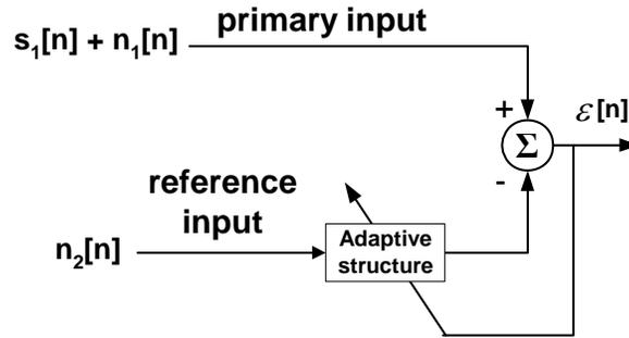
Figure 4 - The adaptive structure used to cancel the slow movement artifacts
