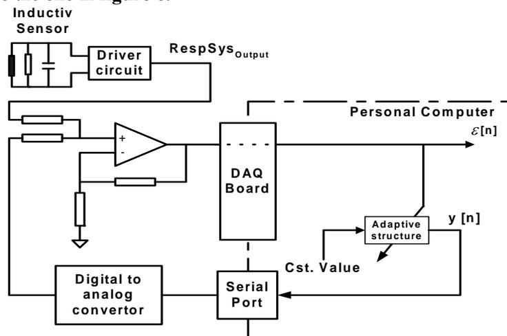
Figure 6 - The second implementation of the adaptive system
