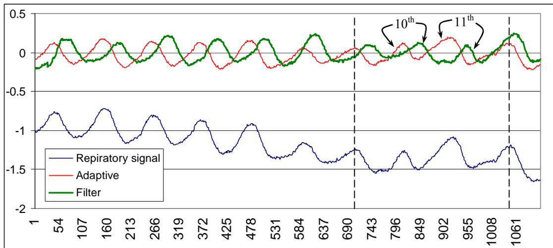
Figure 9 - The respiratory signal affected by artifacts and the two results of the artifacts removing techniques
