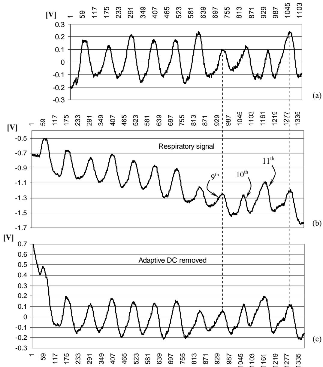
Figure 8 - (a) Resulting respiratory signal using a standard filtering technique (b) The respiratory signal affected by artifact (c) Resulting respiratory signal produced by the adaptive method
