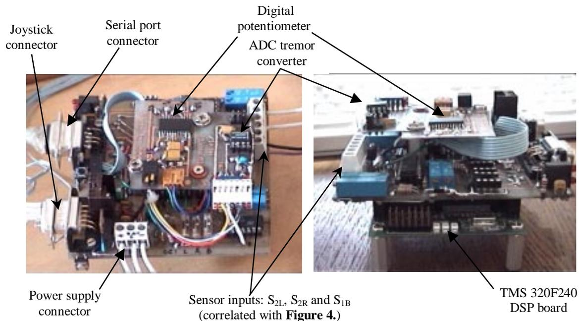
**Figure 3.** Part of the practical implementation of the multimodal virtual joystick
