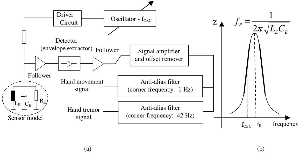
**Figure 2. (a)** Block scheme of circuitry used to drive and control the sensor **(b)** Sensor characteristic
