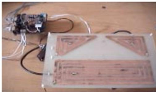
**Figure 1.** 3D Multimodal Interface (the virtual joystick): the sensors and a part of the electronic processing system
