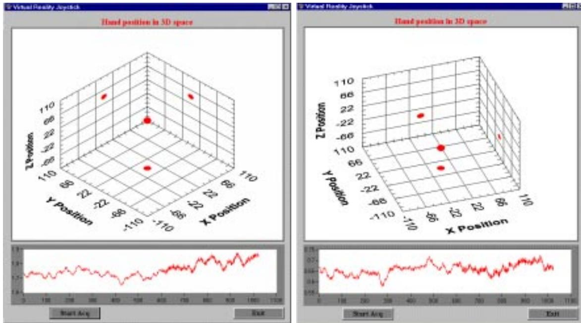
**Figure 5.** Two snap shot with the main window of the PC software program, the red dot representing the hand sensed by the 3D virtual joystick
