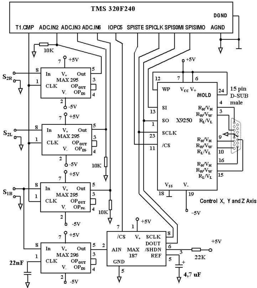
**Figure 4.** Schematics for anti-aliasing filter (for tremor and movement path of the signals), DSP, tremor acquisition converter and digitally-controlled potentiometers
